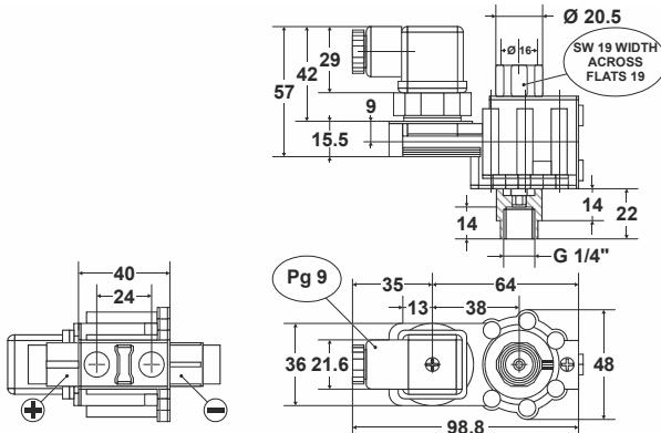
Fig. 6. Dimensions (mm)
