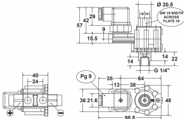
Fig. 2. Dimensions (mm)
