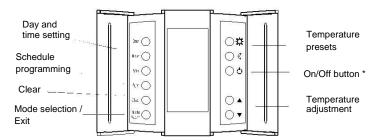
\* Use this button to disable heating (e.g. in the summer). The thermostat remains powered and continues to display the time and temperature.
