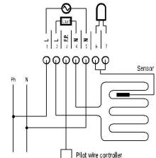
**WARNING:** Ensure that the wires are tightly secured to the terminals. Apply a minimum torque of 0.5 Nm (4.4 Lb/in) when tightening the screws.
