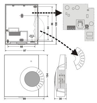
Fig. 3. Dimensions and mounting holes (mm)
