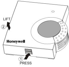
Fig. 2. Cover disassembly
