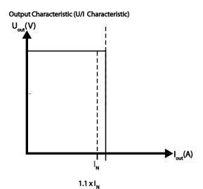
Current overload protection is constant current at (1.1 x nominal current).
