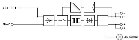
st Two-phase operation only possible if input voltage under 264 Vac.
