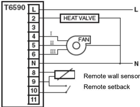
Application 0: Two Pipes, Heating-Only wiring Diagram
